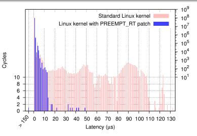
Identify the source of the latency Latency results and comparison
