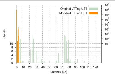
Identify the source of the latency Latency results and comparison
